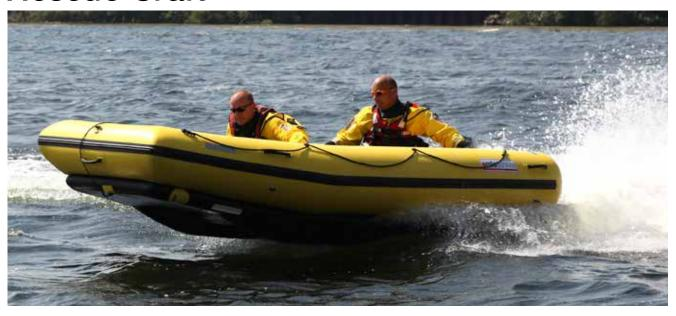
The RC4000 Rescue Craft is designed to exceed the performance of a conventional Inflatable flood rescue boat, while providing the shallow draft and ease of transportation of a rescue sled. The inflatable four meter design with twin keels and a rigid inflatable floor represents the latest thinking in flood rescue boat design.
